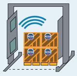
• As the damaged product is loaded on to the truck and passes by the RFID readers at the dock doors, the "impact event" associated with the specific product is automatically entered into the company's warehouse management system.
