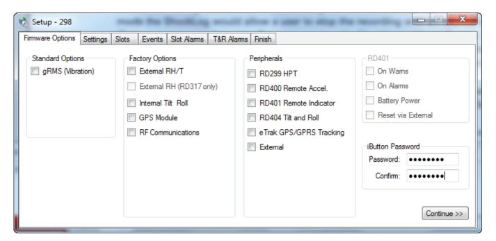
When a ShockLog is programmed with an iButton password, all iButtons used with that ShockLog unit must be programmed with the same password, otherwise the ShockLog unit will ignore the command. To program an iButton with the appropriate password, the iButton must be connected to the PC via the USB connection BUS and then the Password tab selected.
