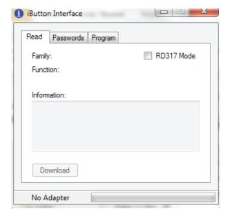
If the user is using an iButton originally set up for the legacy RD317 products, a warning will appear stating that the iButton is for an RD317 and asking "do you wish to change to RD317 mode?" By selecting "Yes", the RD317 mode tick box will be completed and any programming of the iButton will be created in the RD317 compatibility mode.
