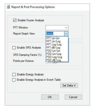
Scroll through the events until the event of interest is displayed. Turn the FFT or PSD analysis on by clicking FFT/PST Off and selecting the desired graph view. FFT Lin/Lin was selected for the image below:
