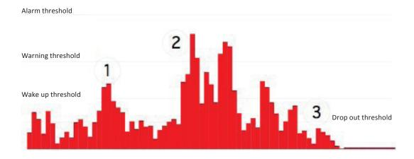
It is not desirable for the ShockLog to constantly be awake due to low level vibration caused by the mode of transport. The ShockLog uses 100 times more battery power when it is recording at higher resolutions than when it is monitoring peak time slot values for wakeup thresholds. The ShockLog can easily see 0.5 to 1g of activity when being transported in a car on normal roads.
