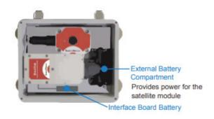
NOTE: Operating the ShockLog Satellite in a location without line of sight to the sky will significantly reduce the battery life of the satellite module.
