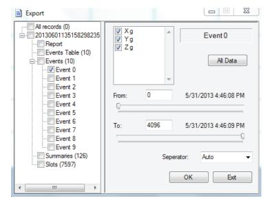
All of these parameters are adjustable. If other events or the slot data on any of the available channels of data is to be downloaded, check the appropriate box. If the entire data file is not of interest but only a proportion is, use the slide bars to adjust the start and finish times of the data to be exported.
